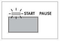
cycle progress is marked by flashing dash under status icon. When appropriate part of drying cycle is accomplished dash becomes steady and appears flashing under next status icon.
